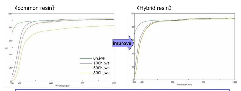
After exposuring, Transmittance down + strength down → Emission trouble, Resin strength down
